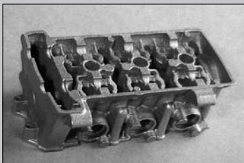
Direct metal laser sintered prototype of a sub-scale cylinder head
